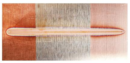
**Fig. 2** This 0.5 mm thick copper sheet prepared with three different surface conditions (etched, oxidized, polished) was successfully welded.
