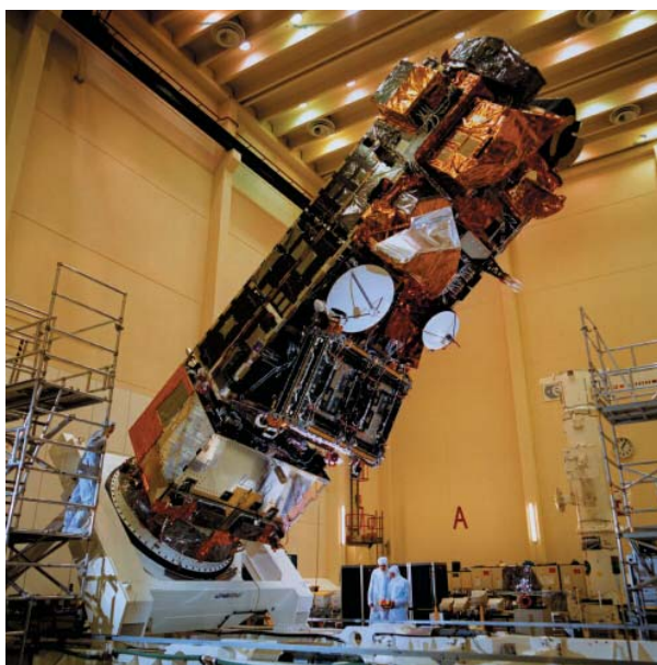
Fig. 1: View of the ENVISAT satellite. Among the experiments MIPAS and GOMOS are dedicated to the study of the terrestrial atmosphere. (Courtesy of M. Endemann, ESA)
