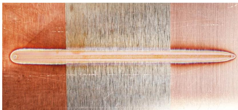
**Fig. 2** This 0.5 mm thick copper sheet prepared with three different surface conditions (etched, oxidized, polished) was successfully welded.
