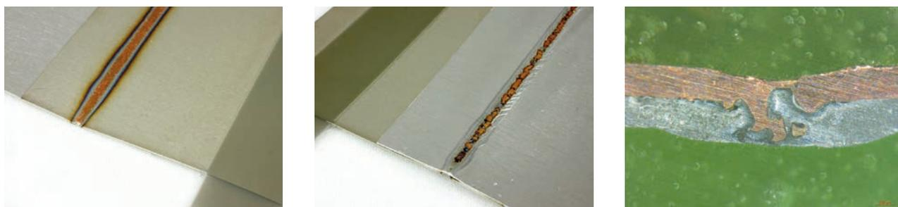
**Fig. 4** Full penetration weld of Ni-coated copper (0.3 mm) to Al sheet (0.3 mm) with  $P = 1000 \text{ W}$ ,  $v = 75 \text{ mm/s}$ .
