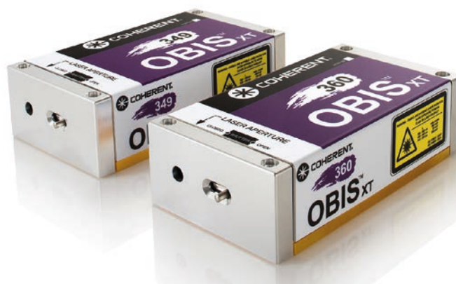
Fig. 2 Two new UV laser wavelengths (349 nm and 360 nm) are now available as part of the OBIS family of compact lasers.
