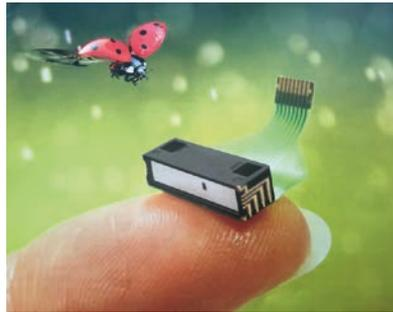
its wavelengths and these are focused on the pixels of the image sensor. The image sensor outputs electrical signals corresponding to the light intensity at each wavelength. Reducing the size of the spectrometer required increasing the curvature of the concave surface and shortening the distance to the image sensor. However, it is extremely difficult to produce a grating on a curved concave surface. Therefore, a return structure consisting of a primary and a secondary reflection mirror is used.
