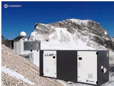
With the aim to extend the height profile of the water vapor concentration into the stratosphere for the first time and thus to investigate its possible influence on global warming, the scientists of the environmental research station Schneefernerhaus on the Zugspitze mountain use a particularly powerful 350-W UV-excimer laser from Coherent. They modified the excimer laser to generate linear-polarized UV pulses with small line width and reduced beam divergence. The re-
