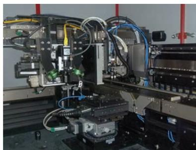
or semiconductor laser dies. – *Selective laser soldering* is the right choice for attaching extremely thin wires to miniature contact pads or insert heat-sensitive components into PCB boards. – *Laser welding* joins two parts without filling material. This joining technology provides maximum mechanical strength and is widely used for space applications. – *Micro ablation* can be integrated into the process flow as an additional inline process.
