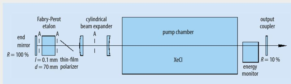
Fig. 2 Scheme of the modified laser system; A: sand-blasted aluminum apertures [4].
