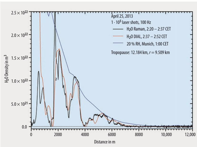
**Fig. 4** Comparison of DIAL and Raman lidar measurements for a strongly layered H<sub>2</sub>O distribution; “Distance” means vertical distance above the lab (2675 m a.s.l.); at two altitudes zero humidity was found by both systems [5]. The differences are explained mainly by atmospheric changes due to a time difference of roughly 15 min between the two measurements. For distances below 1 km the laser beam of the Raman lidar is not yet in the field of view of the telescope.
