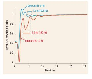
times of 5 to 15 ms are possible. If the distance is not known, the lens can be operated in an oscillatory mode. At low frequencies of, e.g., 5 Hz, several images, each with different working distances, can be captured until a code has been read successfully. While this approach is not particularly fast, it is simple to implement and can be used without calibration.
