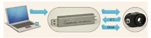
**Fig.3** Control of the variable focal length lens: A USB-based current driver enables accurate control
