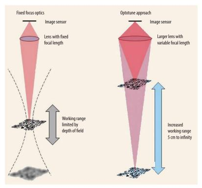
Fig. 2 Difference between optics with fixed focal length (left) and variable focus optics (right)
