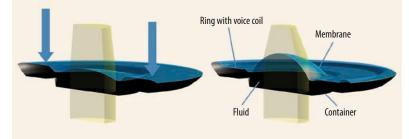
Fig. 1 Principle of operation of Optotune electrically variable focal length lenses: A current-controlled actuator presses fluid through a ring from the
