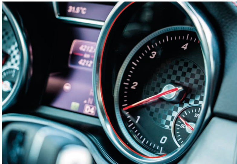
Fig. 6 The glass covers of dashboards need to be welded with precision (position of the weldseam shown in red).
