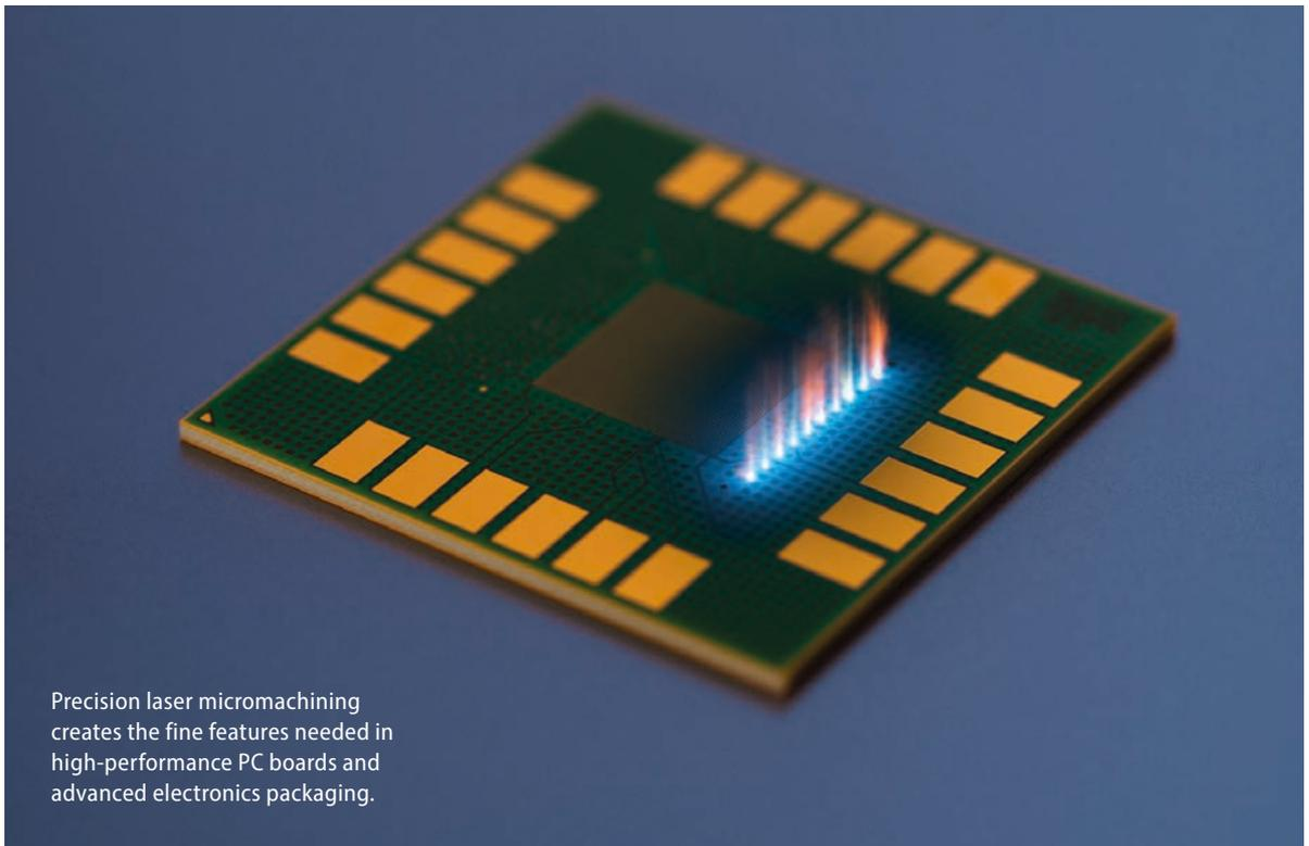
Precision laser micromachining creates the fine features needed in high-performance PCB boards and advanced electronics packaging.
