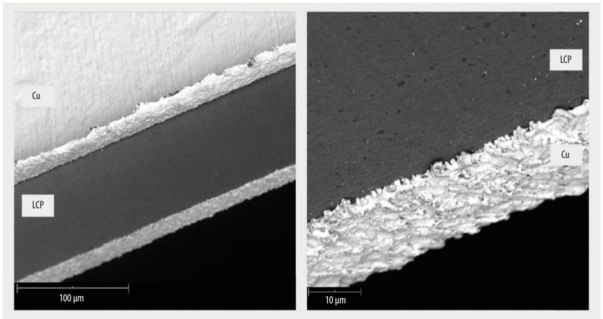
**Fig. 3** SEM imaging reveals smooth material surfaces and crisp geometries of the copper-clad LCP cut with Quasar UV80 laser.
