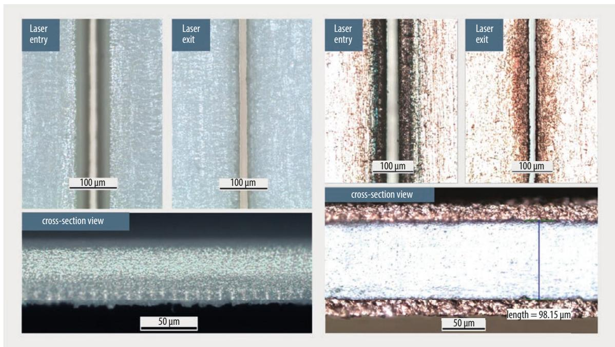
**Fig. 1** Bare 50  $\mu\text{m}$  thick LCP cut with Quasar UV80 laser. Entry (top left), exit (top right), and cross-section (bottom) views indicate excellent quality and minimal excess heating.
