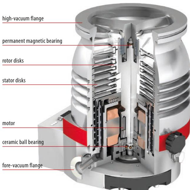
**Fig. 1** Sectional model of a hybrid-bearing turbopump showing the rotor shaft bearing arrangement with a permanent magnetic bearing and a ball bearing.
