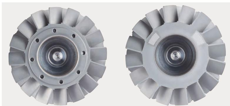
**Fig. 3** Comparison of a balancing level of conventional balancing (left) with balancing holes and of laser balancing (right) with laser ablation segments
