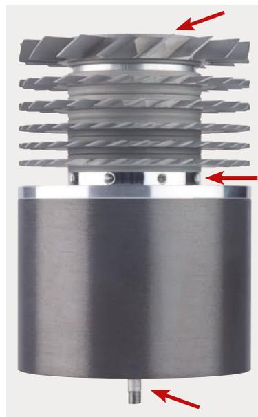
**Fig. 2** Illustration of a turbopump rotor showing the position of the balancing levels.
