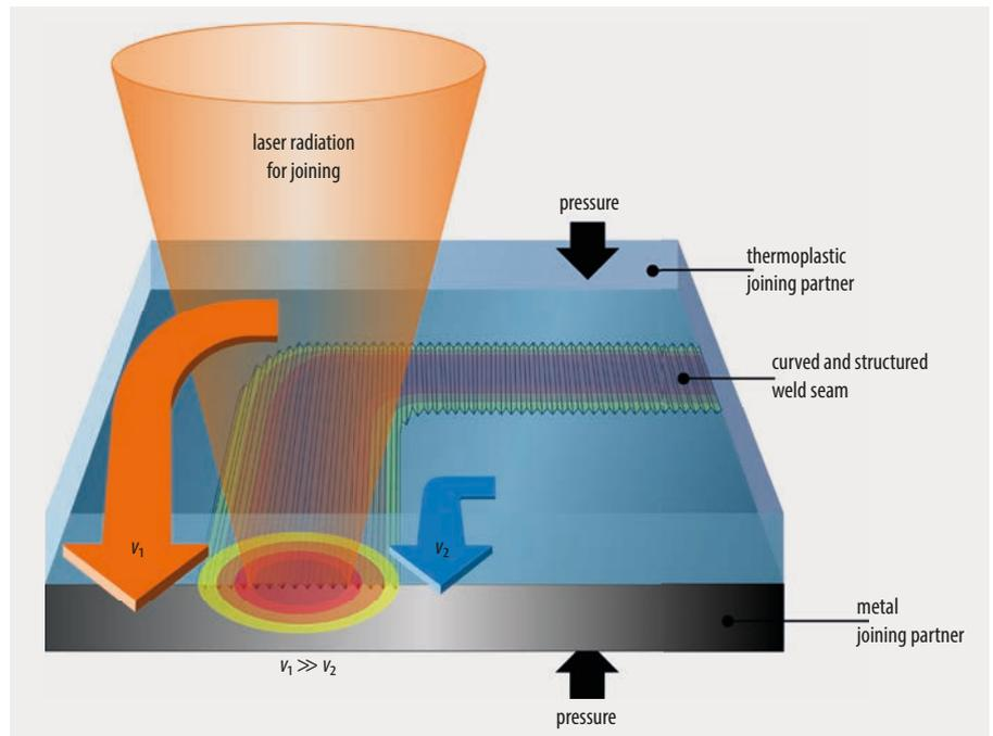
Fig. 1 Heat conduction joining in a curve allows plastic and metal to be melted together.
