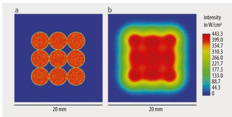
Fig. 2 Spot shape at the focal plane (a) and at the working plane (b), where the spots overlap.
