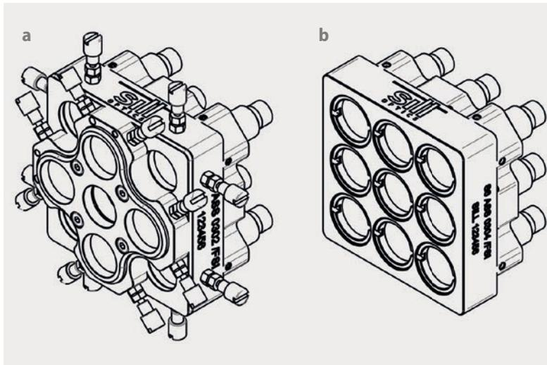
**Fig. 3** A multispot lens is available with (a) and without (b) possible adjustment of the  $x$ - $y$ -position.
