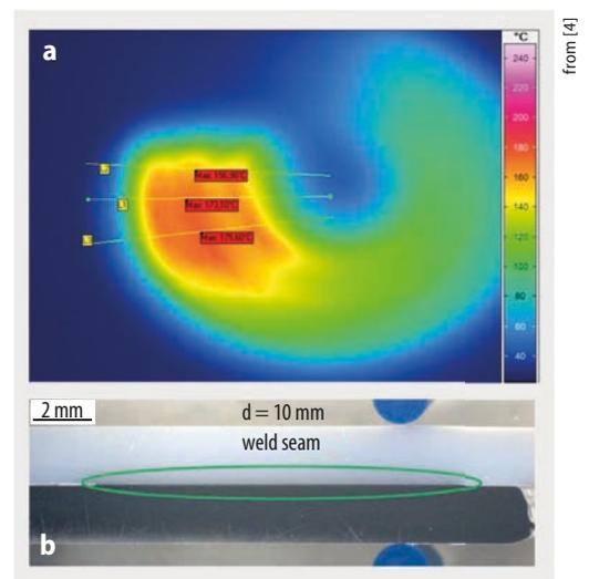
**Fig. 4** A thermal camera (a) proves the optimized energy input at a curve radius of 10 mm. The cross-section of the weld (b) shows its quality.
