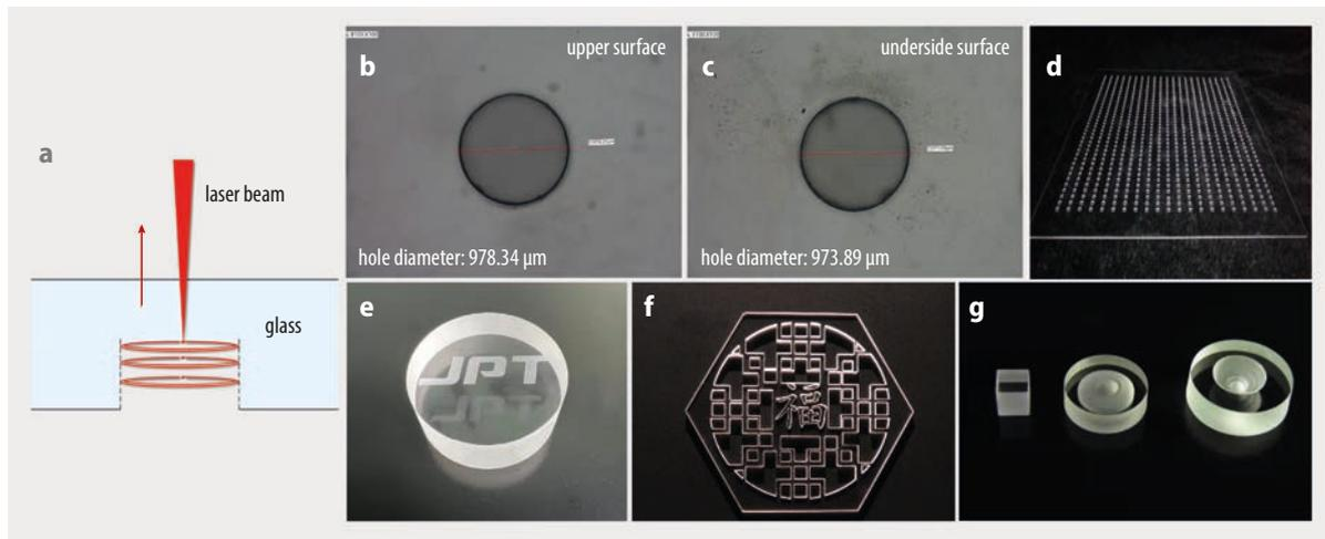
**Fig. 3** The thin red arrow indicates the direction of movement of the laser beam during drilling. Shown are microscopic images of a 1 mm hole drilled in substrate glass (b, c) and images of laser drilled samples, including through holes and blind holes (d – g).
