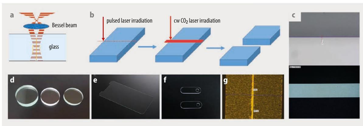
**Fig. 2** The focal depth of a Bessel beam (a) can reach several millimeters. It is used for the cutting and splitting process of brittle material by an ultrafast laser (b). Shown are cross-sectional microscopic images (c), circular cuttings of thick glass (d), special-shaped cutting of cover glass (e) and camera (f) and laser cutting of double laminated glass (g).
