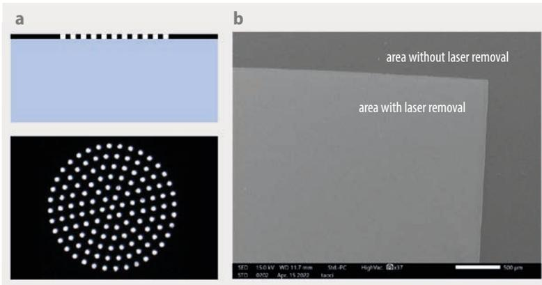
**Fig. 4** UV picosecond lasers can remove deco (a), the black color indicates the deco layer. The image of functional thin film removal on glass (b) was taken by a scanning electron microscope.
