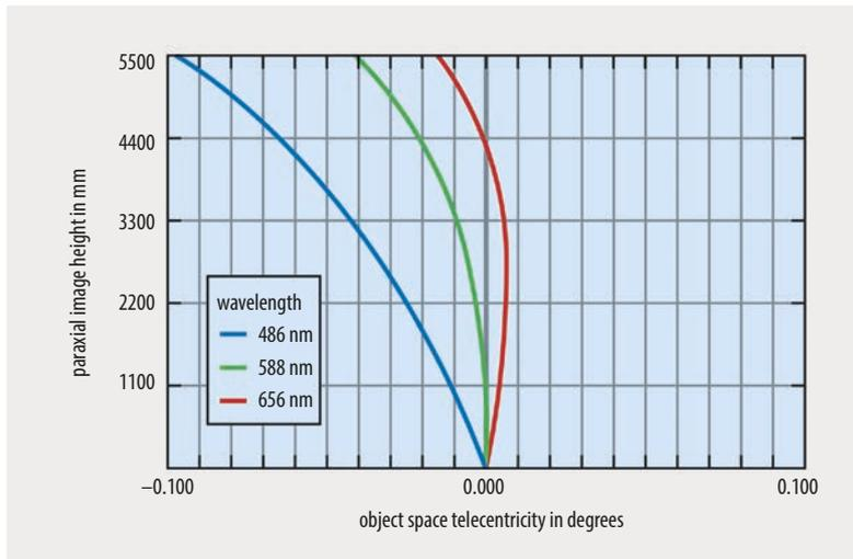
**Fig. 3** The example of a 1X lens shows that image height and telecentricity depend on each other differently at varying wavelengths.
