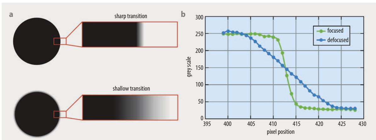
**Fig. 2** A telecentric lens depicts a point differently measured in focus (a, above) or with a slight defocus (below). The effect of defocus is distributed symmetrically. The course of the grey scale (b) shows that the edge is distributed over several pixels in the defocused case (blue), which can lead to more repeatable results than in the focused case (green).
