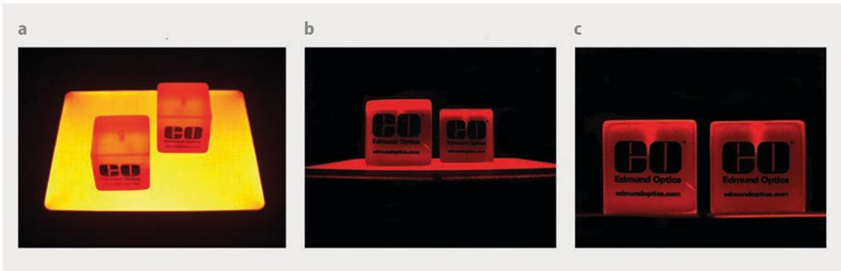
**Fig. 1** The two cubes are identical, but have different distances to the camera (a). Due to the aperture angle of the fixed focal length lens, the right cube is imaged smaller than the cube that is closer to the inspection system (b). In the same scene taken with a telecentric lens both cubes are the same size (c).
