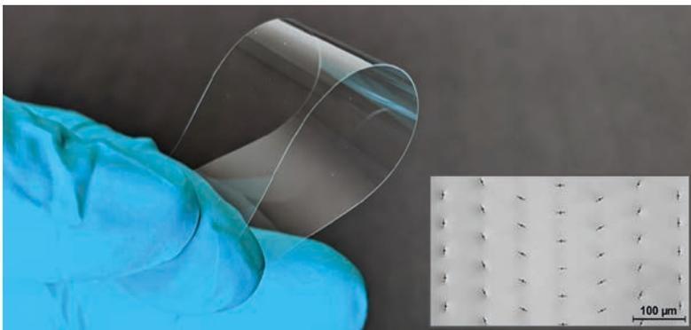
**Fig. 3** The ultrathin glass, separated by an optical concept generating multiple Bessel-like beams. The inset shows a reflected light microscope image of the laser-induced changes/cracks from above. From left to right, the orientation of the beam profile was changed in  $30^\circ$  steps. It shows that the alignment of the applied cracks can be controlled by aligning a Bessel-like beam with two local intensity maxima [3].
