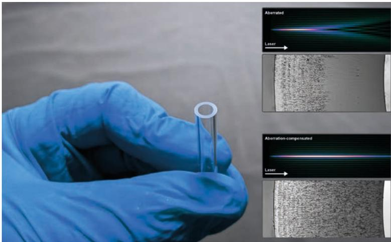
**Fig. 4** The glass tube is cut by an aberration-corrected laser beam. The upper inset shows the longitudinal intensity distribution aberrated by the curved surface and corresponding material modification. In the lower inset the aberration is corrected [5].
