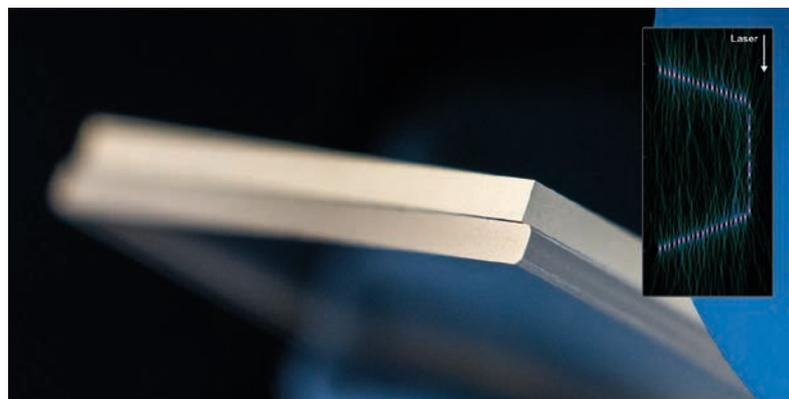
**Fig. 5** The 550  $\mu\text{m}$  thick Gorilla glass sample has a modified 45° edge geometry generated with a single laser pass. The inset shows the holographic intensity distribution of several dozen nearly ideal single spots in a plane perpendicular to the glass surface and to the feed direction [6].
