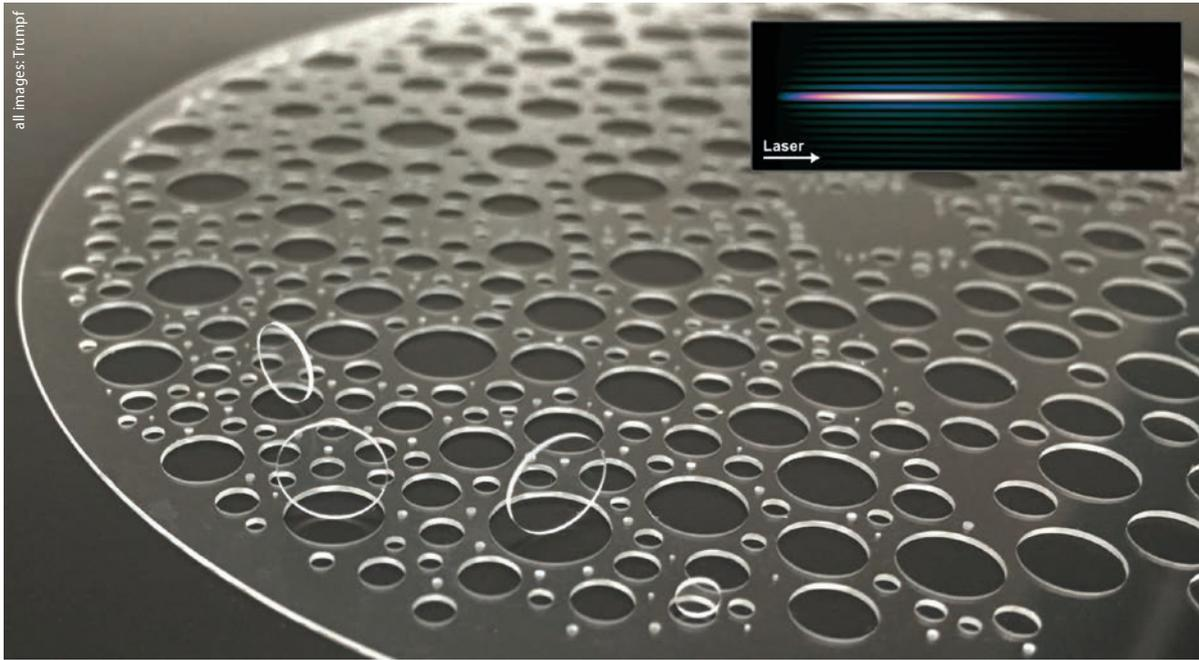
**Fig. 1** The inner contours were cleaved using a TruMicro 2030 ultrashort pulse laser beam shaped into a Bessel-like intensity distribution with TRUMPF TOP Cleave-2 optics (inset) [4].
