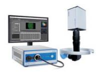
Thanks to its innovative one-shot process, the VTC infrared camera simultaneously measures the spatial polarization of the individual emitters of a VCSEL array and delivers the information necessary to reduce the polarization dependence of the measurement setup. This procedure minimizes the error budget of the VCSEL
