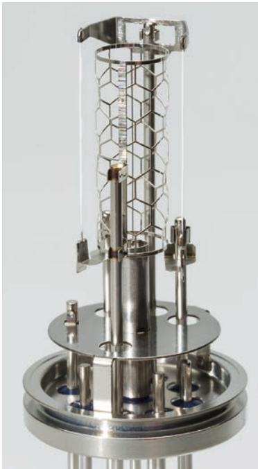
Fig. 2 An example of a Bayard-Alpert hot-filament ionization gauge
