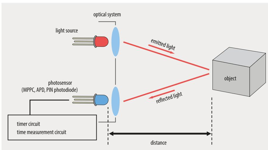
In automobiles, lidar mainly uses the direct time-of-flight method: The distance corresponds to the time duration a light pulse needs to travel from the source to an object, to be reflected, and to return to the sensor.
