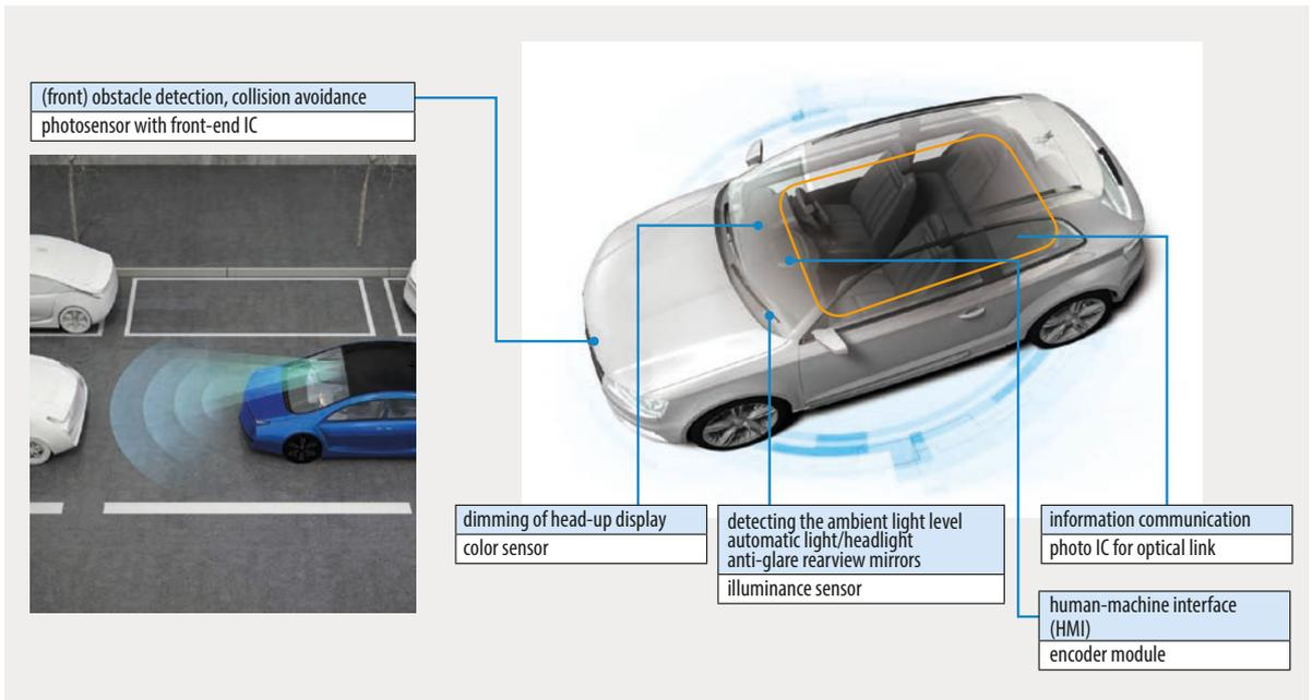
The photosensor with front-end IC optically measures the distance to the front car return and controls the distance to the vehicle.
