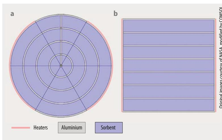
**Fig. 5** In these designs for cylindrical (a) and rectangular beds (b), the sorption surface, the distance between the aluminium/steam chambers and the length of the heater remain unchanged.
