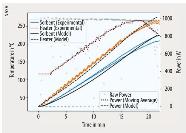
**Fig. 4** The experimental results from the focused test and the thermal model show good agreement.
