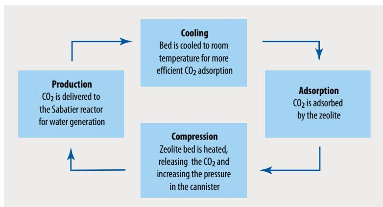
**Fig. 2** The complete cycle for pressurising the CO<sub>2</sub> in the AC-TSAC process takes 150 minutes.
