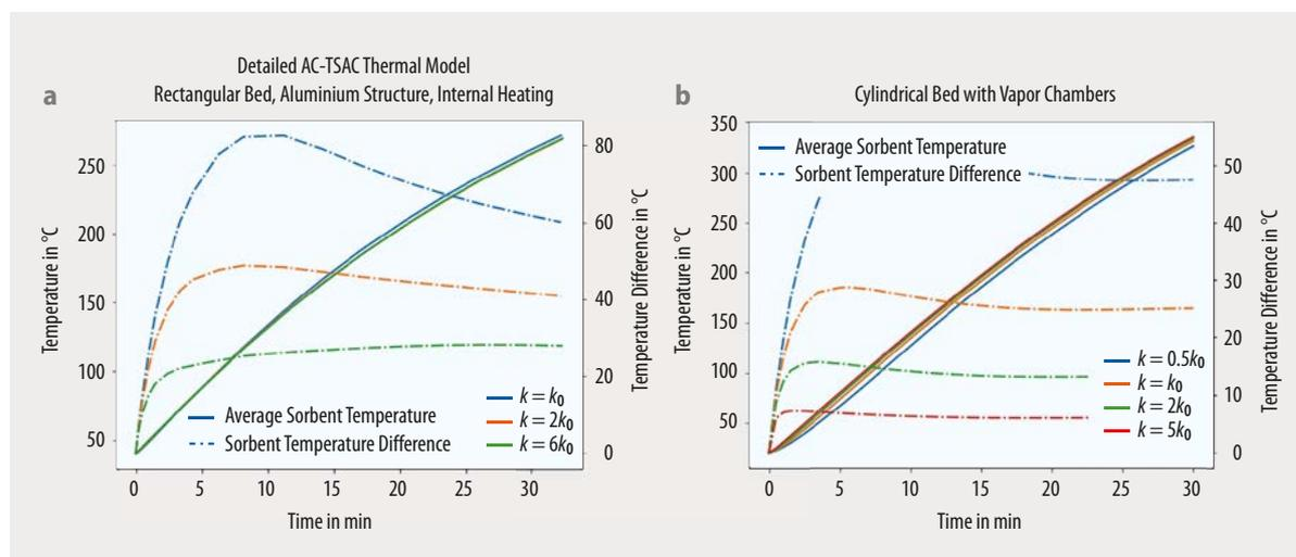
**Fig. 6** Increasing the thermal conductivity ( $k$ ) leads to less of a temperature difference of the sorbent throughout the bed.
