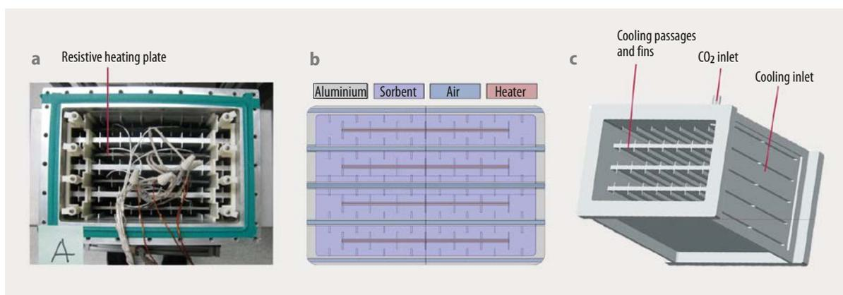
**Fig. 3** The actual compressor (a) can be easily visualised using both a 2D model (b) and a 3D model (c). A 2D model was therefore sufficient for further modelling.
