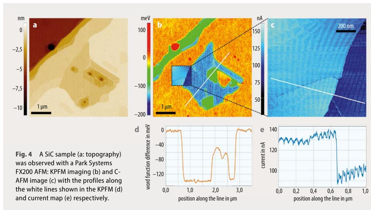
**Fig. 4** A SiC sample (a: topography) was observed with a Park Systems FX200 AFM: KPFM imaging (b) and C-AFM image (c) with the profiles along the white lines shown in the KPFM (d) and current map (e) respectively.
