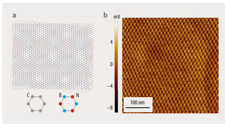
**Fig. 1** The relative twist between superpositioned graphene (grey) and hBN (blue/red) layers results in a honeycomb moiré pattern (a). The measurement of the LFM map of graphene/hBN with a Park Systems FX40 AFM shows a moiré pattern in the lateral deflection signal (b).
