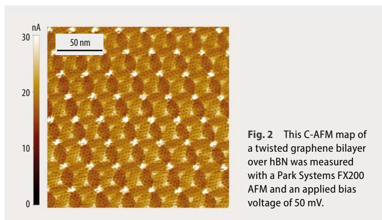
**Fig. 2** This C-AFM map of a twisted graphene bilayer over hBN was measured with a Park Systems FX200 AFM and an applied bias voltage of 50 mV.
