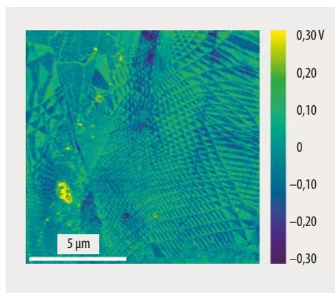
**Fig. 3** This KPFM image of the surface potential of a hBN bilayer over graphene was measured with a Park Systems NX20 AFM.
