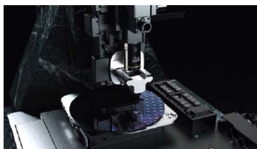
Fig. 2 In this close-up of the AFM, the AFM head can be seen in the center above a wafer sample. On the left side are the two cantilever cassettes, which can hold up to 16 different cantilevers.
