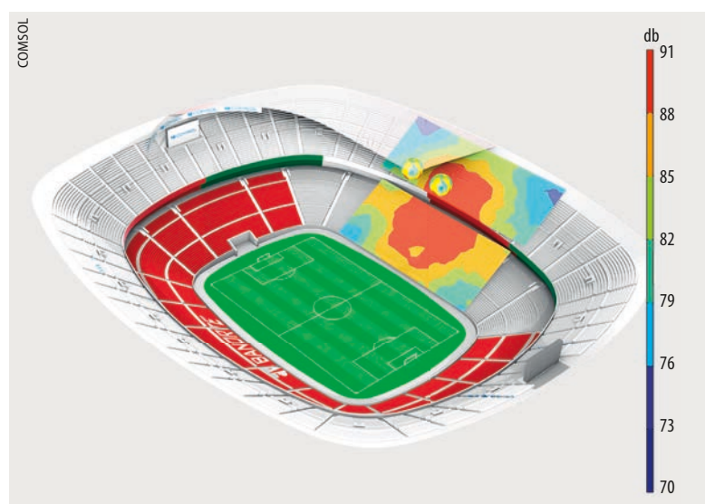
Fig. 4 A sound-pressure-level map reveals the acoustic field in a plane above the seating area and below two loudspeakers.
